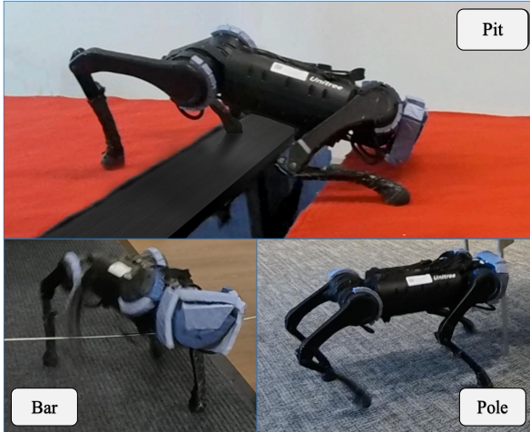
Fig. 1: Our Robust Robot Walker is passing through various challenging “tiny traps” including Pit, Bar, and Pole solely relying on its proprioception by single policy.
