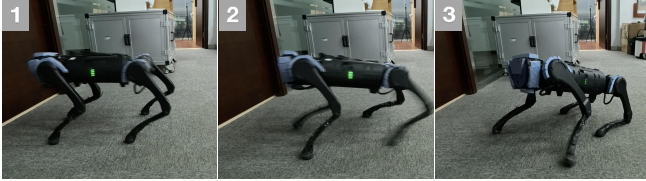
Fig. 9: The robot falls down on the ground with boolean value estimation. While using encoded contact force as estimation value, the robot can continually change the speed with a minimal sim-to-real gap, as shown in appended video.
